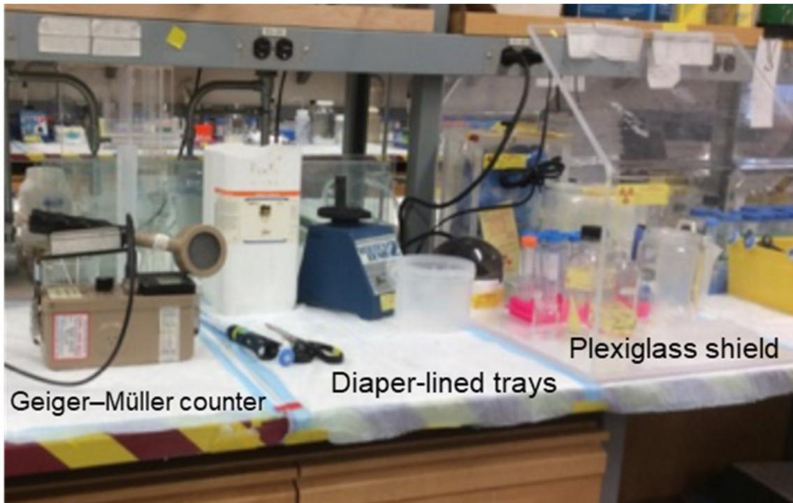
Figure 3: Example of a radioactive working area
