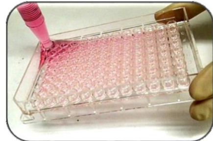
Easy one step media exchange by tilting the plate and aspirating from the corner.
